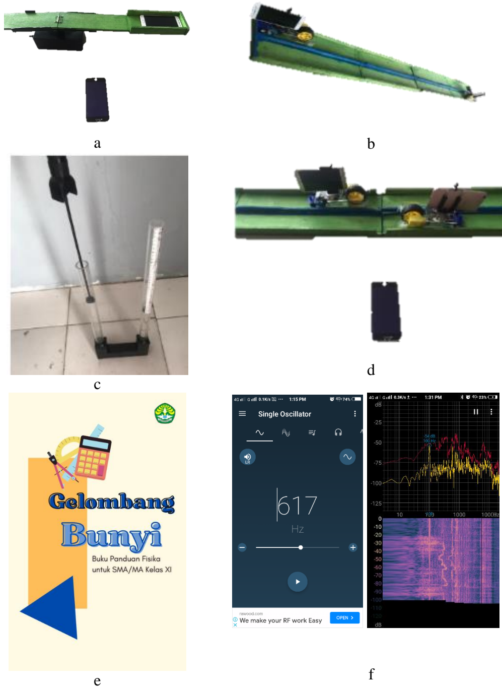
Figure 2. a. Rotational Doppler Effect Experiment Set, b. Linear Doppler Effect, c. Resonance, d. Drifting, e. Instruction Manual, f. Frequency Generator and Spectroid Application
